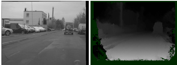
Figure 3. Van scene (rectified left image shown on the left) and corresponding disparity scene (right). Here, SGM with BT is used. The cameras deliver 12 bits per pixel and have a 55cm baseline with a 26^\circ field of view. Dark green marks unmatched areas.
