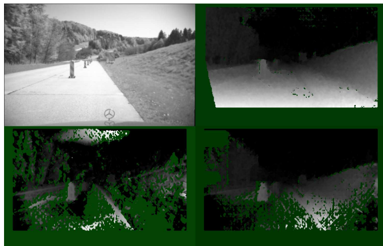
Fig. 7. Resulting Disparity Maps for the Construction Site Scene (top left). SGM with ZSAD (top right) works well while SGM with BT (bottom left) and SGM with HMI (bottom right) fail. The image pair has a strong vignetting effect and different brightness. Small disparities are mapped to black, invalid pixels are marked dark green.
