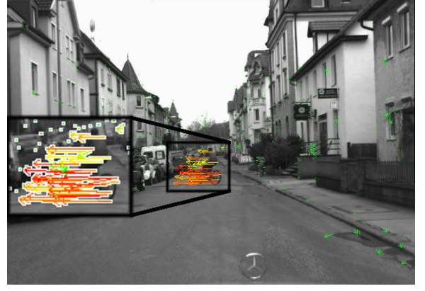
Fig. 7. Velocity estimation results with image based ego-motion compensation.
